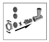
First, place the screw shaft with plastic seal inside the screw housing. Place the knife on the screw shaft with the flat surface facing out.
